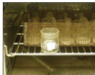
The sample is dried in an oven at 105°C for 90 min.
