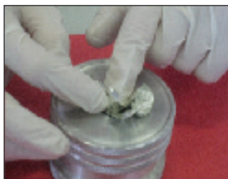
The tin disk is closed by hand using the capsulator.
