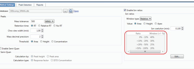
Figure 2. ToxFinder data processing method. Compounds are identified based on retention time and ion ratio. Ion ratio accuracy criteria are specified in the method table.
