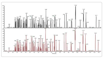
Using the Instant Connect Helium Saver Module, results from US EPA Method 8270C (semi-volatiles) remain unchanged
