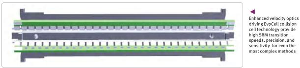
driving EvoCell collision cell technology provide high SRM transition speeds, precision, and sensitivity for even the most complex methods
