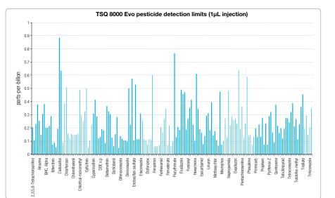
The TSQ 8000 Evo GC-MS/MS is a perfect fit for laboratories in need of high efficiency pesticide methods. Enhanced selectivity, speed, and sensitivity translate into real routine efficiency and productivity. Expect performance above and beyond former triple quadrupole instruments.
