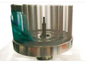
Screen capture of vial in quick spin shaking mode
