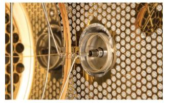
GC oven view with direct column connection to the TriPlus 500 HS autosampler
