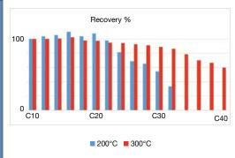
Long Sequence Area Counts Repeatability. 120 consecutive headspace injections of a 50 ppm ethanol solution in water (5 ml in 10 ml crimp top vial). Overall RSD%=0.7. Recovery of a standard hydrocarbon mixture C10-C40 at high temperature operation, showing >60% recovery at 300°C
