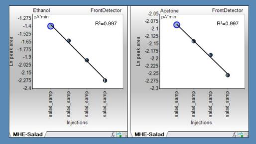
MHE linearity for ethanol and acetone in salad wrap sample. For both the analytes, the resulting correlation coefficients ( $R^2$ ) are extremely good, assuring accurate quantitative results.
