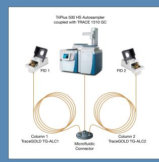
Dual-FID configuration implemented through a microfluidic connector
