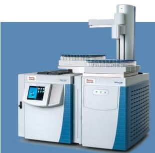
TriPlus 500 HS autosampler (240-vial configuration) connected to the TRACE 1310 GC. The highest sample throughput in the most compact design.
